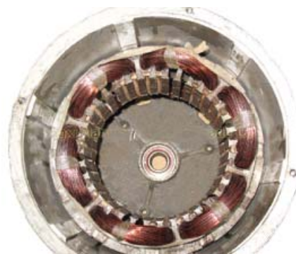
Generator stator coil
